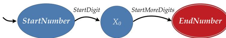
**Figure 2.7. Converting the *Number* productions to an RTN.**
