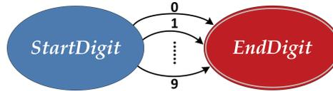
**Figure 2.9.** Converting the *Digit* productions to an RTN.
