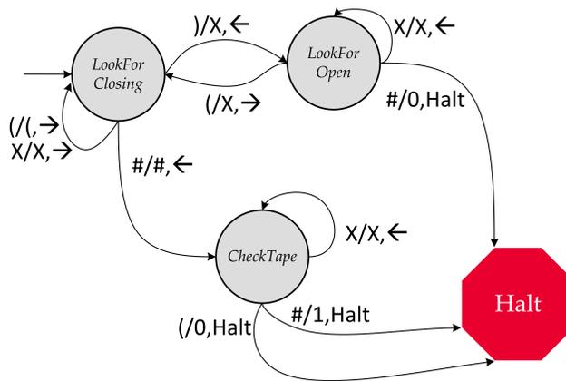
Figure 6.8. Checking parentheses Turing Machine.
