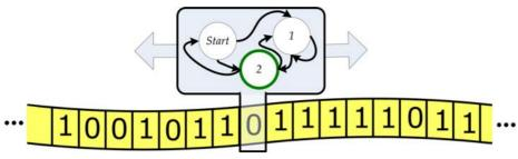
Figure 6.4. Turing Machine model.
