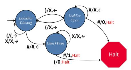
Figure 6.6. Checking parentheses Turing Machine.
